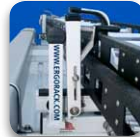
THE PADDED, ADJUSTABLE AUTO-CLAMP (FRONT CROSSBAR ONLY) LOCKS LADDER IN PLACE WHEN STOWED TO REDUCE VIBRATION AND ENHANCE LADDER LIFE
