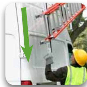
SLIDE EXTENSION LOWERS THE LADDER FOR EASY UNLOADING OR LOADING.
