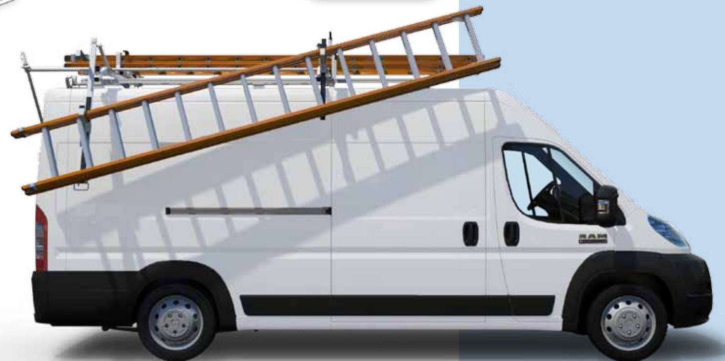
THE PADDED, ADJUSTABLE AUTO-CLAMP (FRONT CROSSBAR ONLY) LOCKS LADDER IN PLACE WHEN STOWED TO REDUCE VIBRATION AND ENHANCE LADDER LIFE
